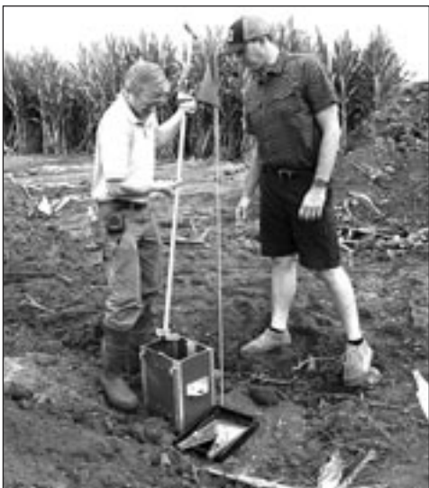
Ryan Arch, ILCA, and Ethan Koehler, farmer, show how water samples are taken to calculate the efficiency of the bioreactor. ( www.ilfb.org )
